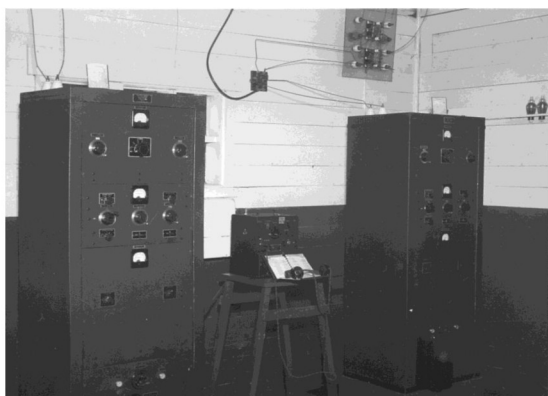
Figure 4. Two Standard Electric ITG200 transmitters used on Marion Island during the 1950's. They stand on plinths as the old radio hut was built on very marshy soil and had wooden walls, covered with corrugated iron panels; it had a raised wooden floor. (Picture sourced from Stellenbosch University, Antarctic Legacy Archive.)
