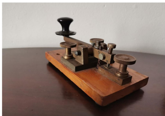
Figure 3. Skirted knob PATT.1056.A. Morse key used on Marion Island during the 1950's.
