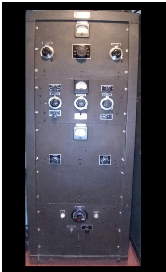
Figure 5. Five rack-mounted units complete the ITG200 transmitter. A terminal strip in the rear of the rack allows connection of microphone, CW key and remote control.
