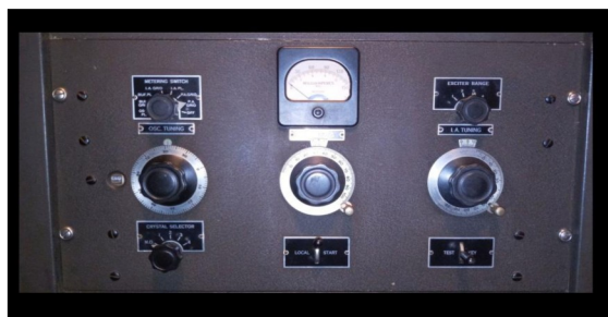
Figure 6. Exciter front panel of the ITG200. The VFO dial is to the right, followed by the intermediate stage and final stage tuning. Adequate metering is available to adjust and monitor all stages.
