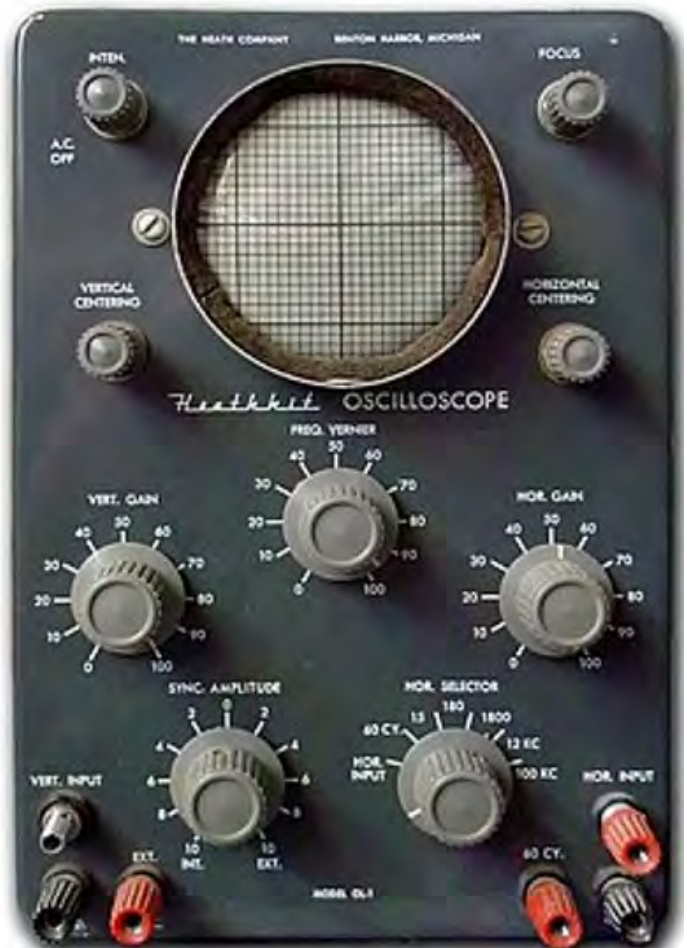
An oscilloscope OL-1 from 1954, the company's first with a relatively small 3-inch CRT which allowed for a highly competitive price of US$ 29.50 (equivalent to $354 in 2025) for the DIY kit. 1
