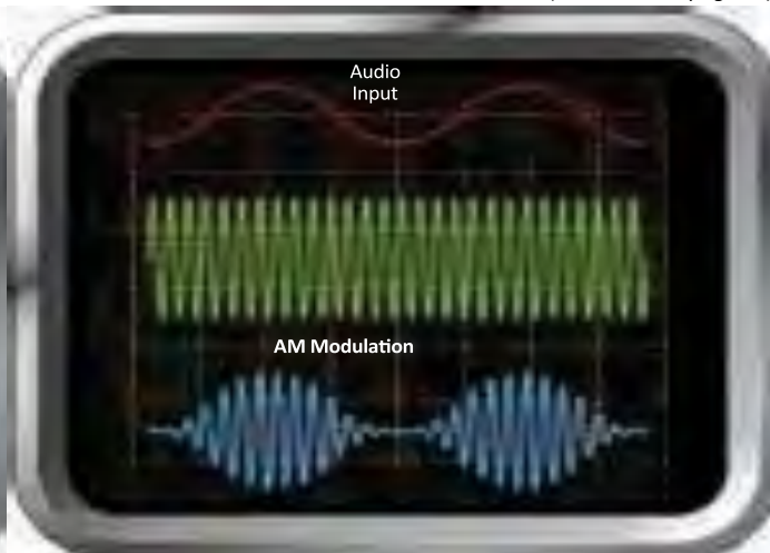
In AM modulation, the carrier frequency remains constant and the signal amplitude changes.
