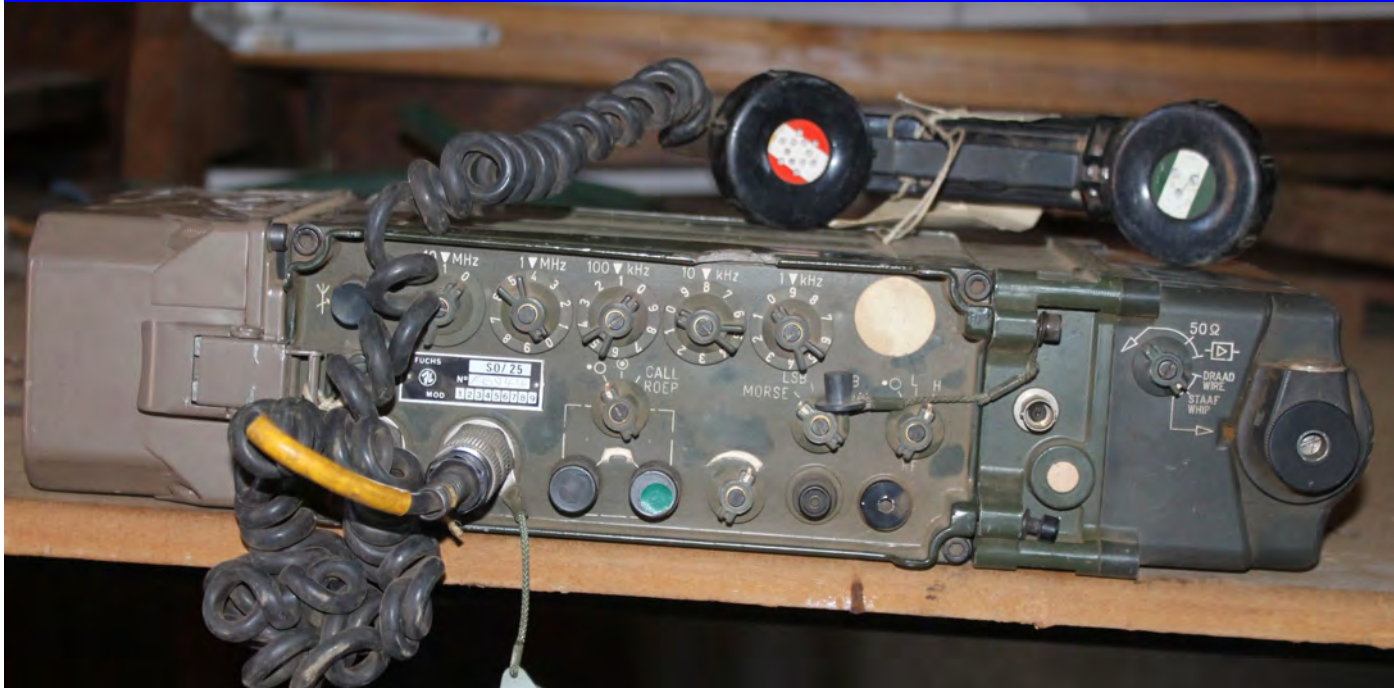
The RS B25 SA Manpack radio as used by the Infantry. On the left, the battery; middle the transceiver and right the Antenna Tuning Unit
