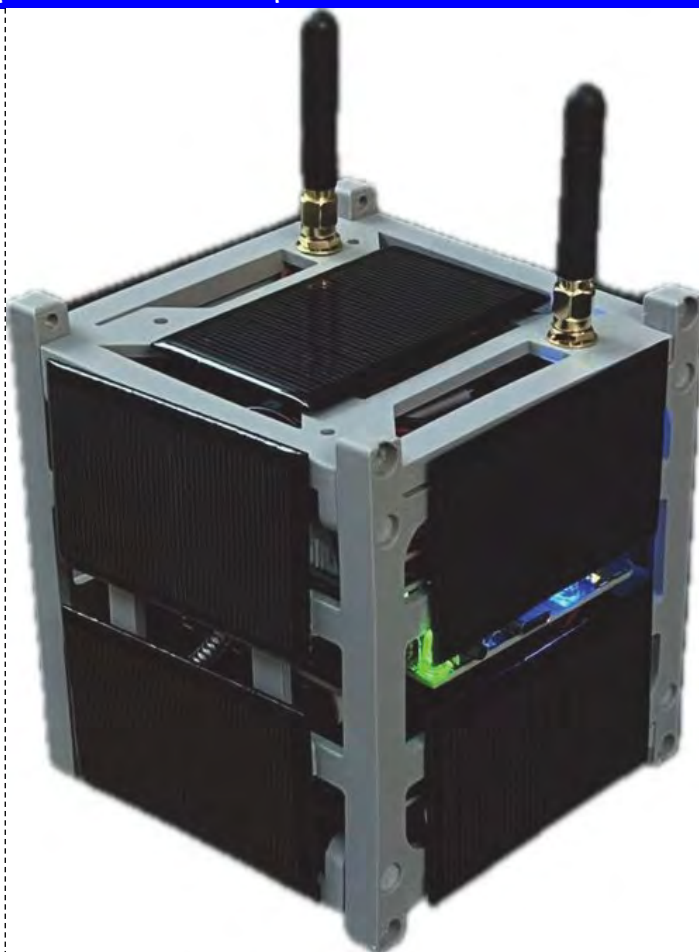
The fully assembled AMSAT CubeSatSim. [Photo courtesy of Mark Samis, KD2XS]
