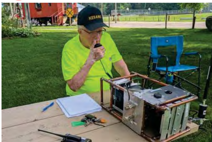
The ARISS STAR XRP Rover, with a CubeSatSim Lite installed. This device allows students to simulate NASA Mars rover operations; the attached CubeSatSim serves as an SSTV camera and it can also be used as a cross-band repeater. [Mark Samis, KD2XS, photo]
