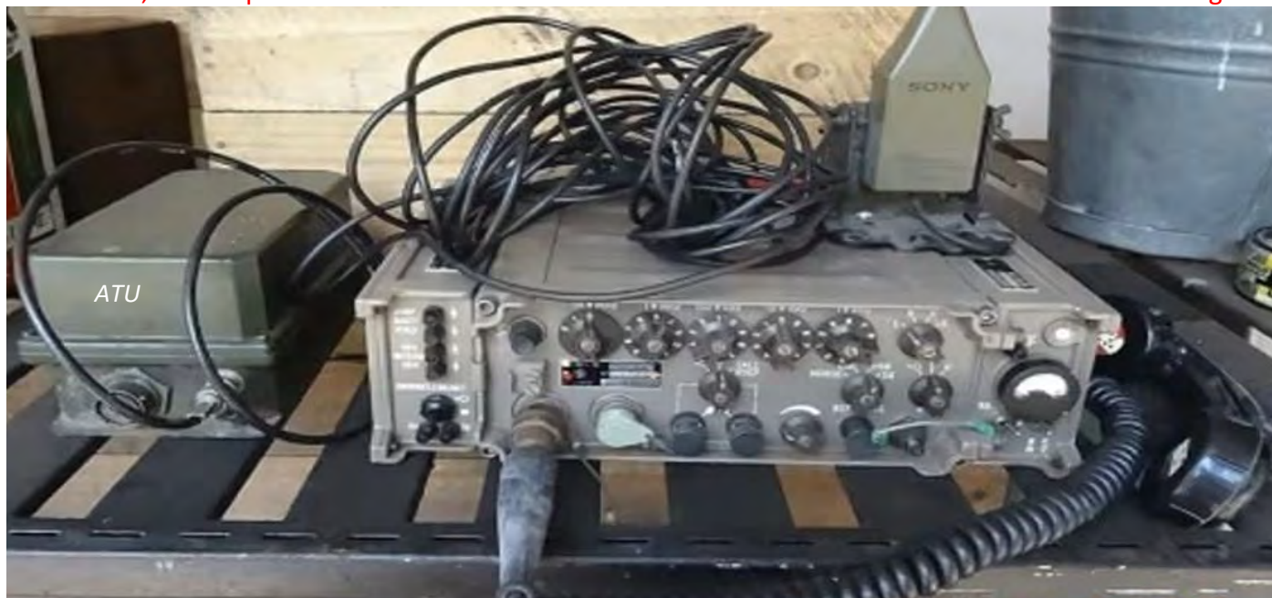
The RS B26 SA Vehicle radio. On the left, the Power Supply Unit; middle the transceiver and right the Antenna Control Unit. The ACU is connected to the ATU by coax cable and a multi-wire control cable.
