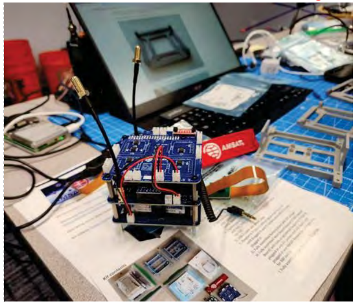
The PCB stack for the no-solder CubeSatSim kit, consisting of a main board, solar board, battery board and a Raspberry Pi Zero 2 W, assembled during a 2025 ARRL Teachers Institute on Wireless Technology (TI) Space Comms and Radio Astronomy session. [Matt Severin, NSMS, photo]
