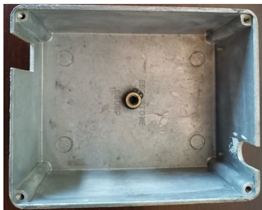
Fig 3: The Eddystone dust cover protects the components of the key, as well as the operator. No wiring is exposed. The cover is easily removed for key cleaning, adjustment or inspection. These covers have Eddystone 6908P print moulded into the reverse side of the cover top.
