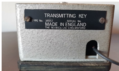
Fig4: Name tag of the type No 365FZ key. The diecast aluminium box is painted a metallic grey.
