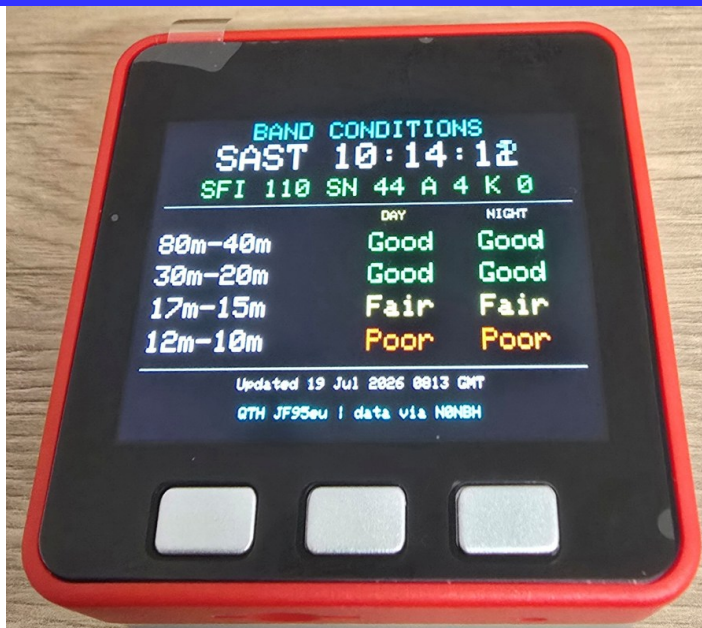
Figure 1. The completed dashboard running on the M5Stack Fire.
