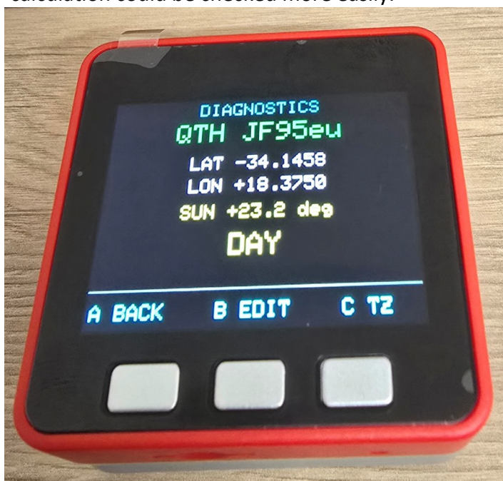
Figure 3. Maidenhead coordinates, solar elevation and the resulting daylight decision
