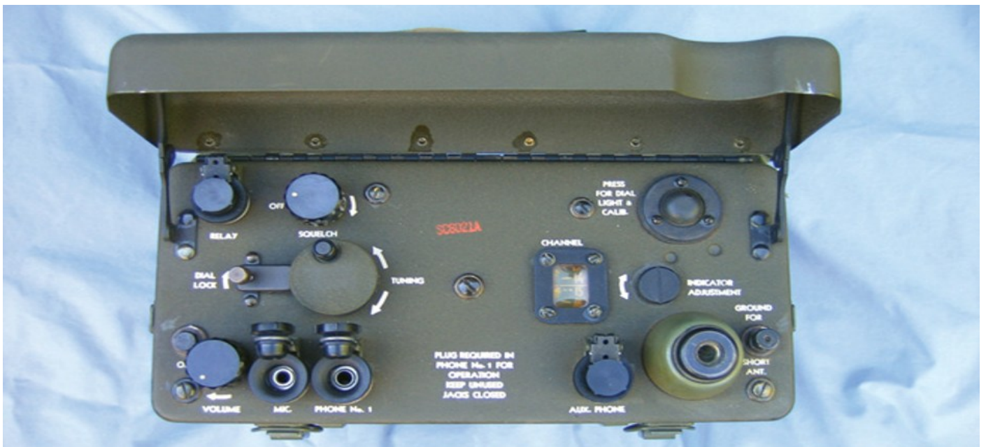
The control panel of the BC-1000 transmitter/receiver, with the hinged cover up
