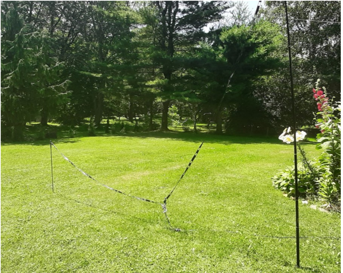
(A 5-Band, Lazy-L, Linear-Loaded, Ladder Line Antenna from page 68)
