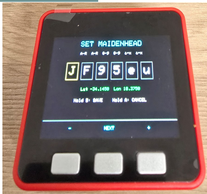
Figure 4. The on-device six-character Maidenhead editor and decoded position
