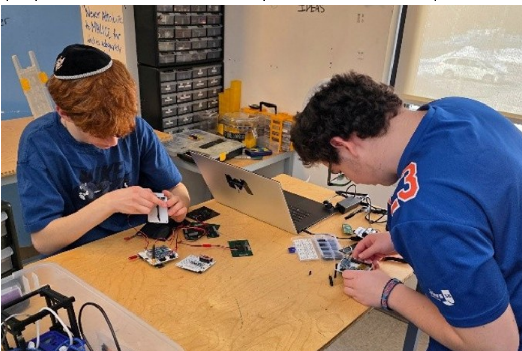
Leffell School Space Engineering Programme students assemble the AMSAT CubeSatSim. [Raz Idan, KE2FEB, photo]
