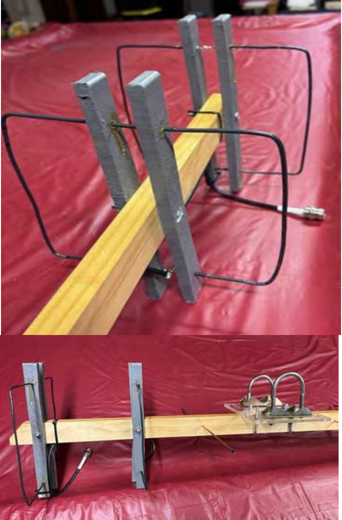
Figure 3. The Quagi with a cross-boom mount. [Richard Lawn, W2JAZ, photo]
