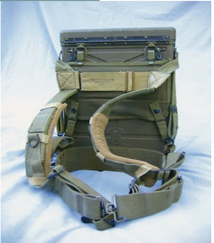
The harness attached to the BC-1000 radio unit is imprinted with "Mid-West Duck & Canvas Co 1943." Note the thick felt pads that have been slipped over the shoulder straps. The felt cushioned the shoulders, vastly improving the comfort of the harness.
