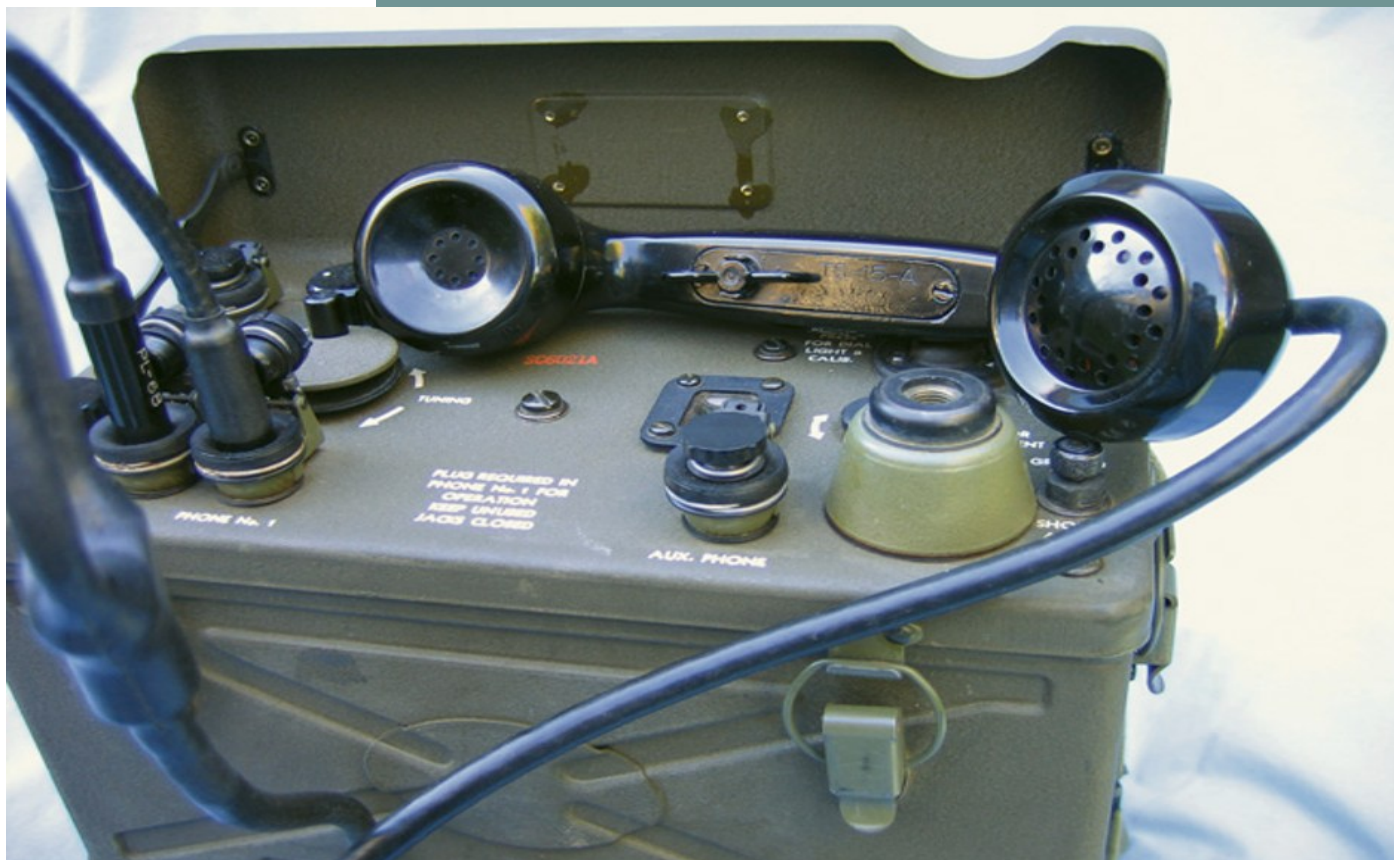
The telephone-like Handset TS-15-A. Note the “butterfly” switch that, when rotated either direction, activated the transmit circuit.
