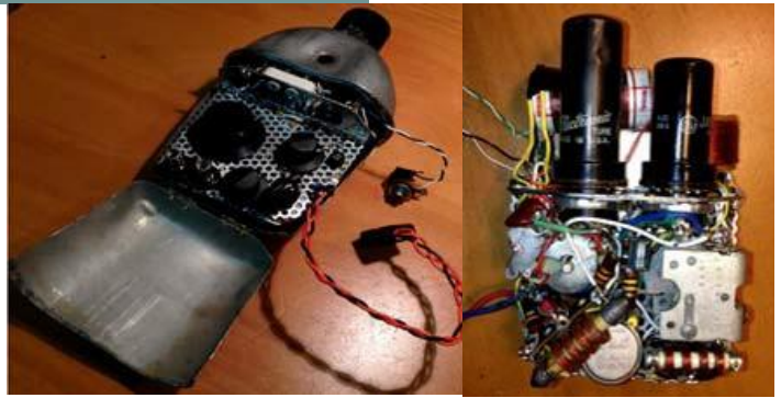
Author's two-tube canteen transceiver
