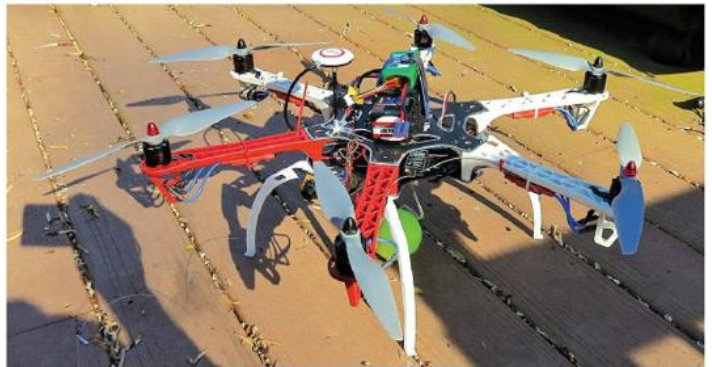
Figure 1. The drop drone, a OJI F550 Flamewheel Hexacopter, in pre-flight position.
