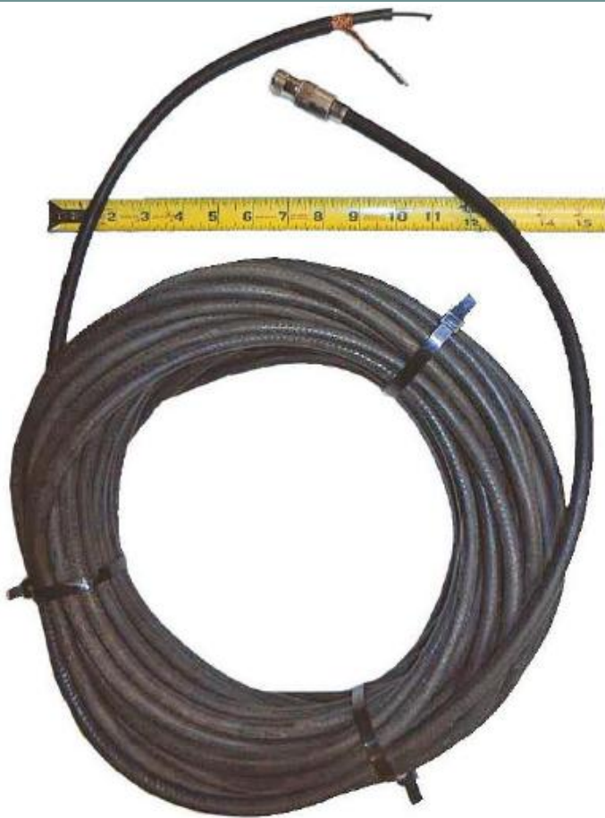
Figure 2. The matching stub is an 88-foot, 8-inch-long piece of RG-11 75 Ω coax, wound tightly into a choke configuration and held in place with wide nylon zip ties.
