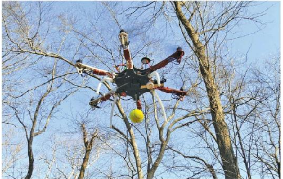
Figure 2. The drop drone, a OJI F550 Flamewheel Hexacopter, after liftoff. Note that the trailing line is too thin and translucent to show up in the photograph.
