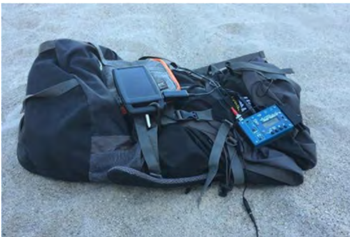
A compact portable CW station used on Santa Rosa Island, featuring an MTR-3B QRP transceiver, a Palm Morse Code paddle and a lightweight portable battery. This minimalist setup highlights efficient, low-power CW operating from a remote island location. Photo by Philomen Leonelli Jr., WM6Y.
