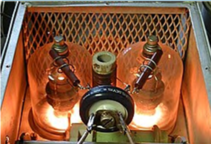
Above. Glowing cathodes in two transmitting vacuum tubes
