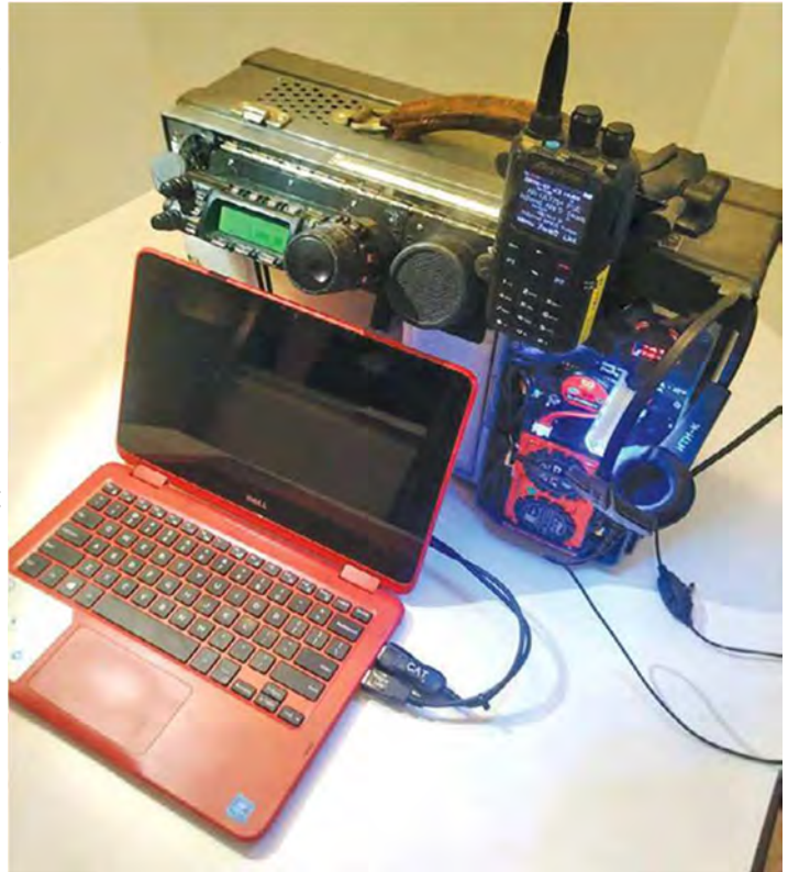
This all-band go-kit includes a radio, antenna tuner, laptop, battery management system, accessories, safety features and more.
