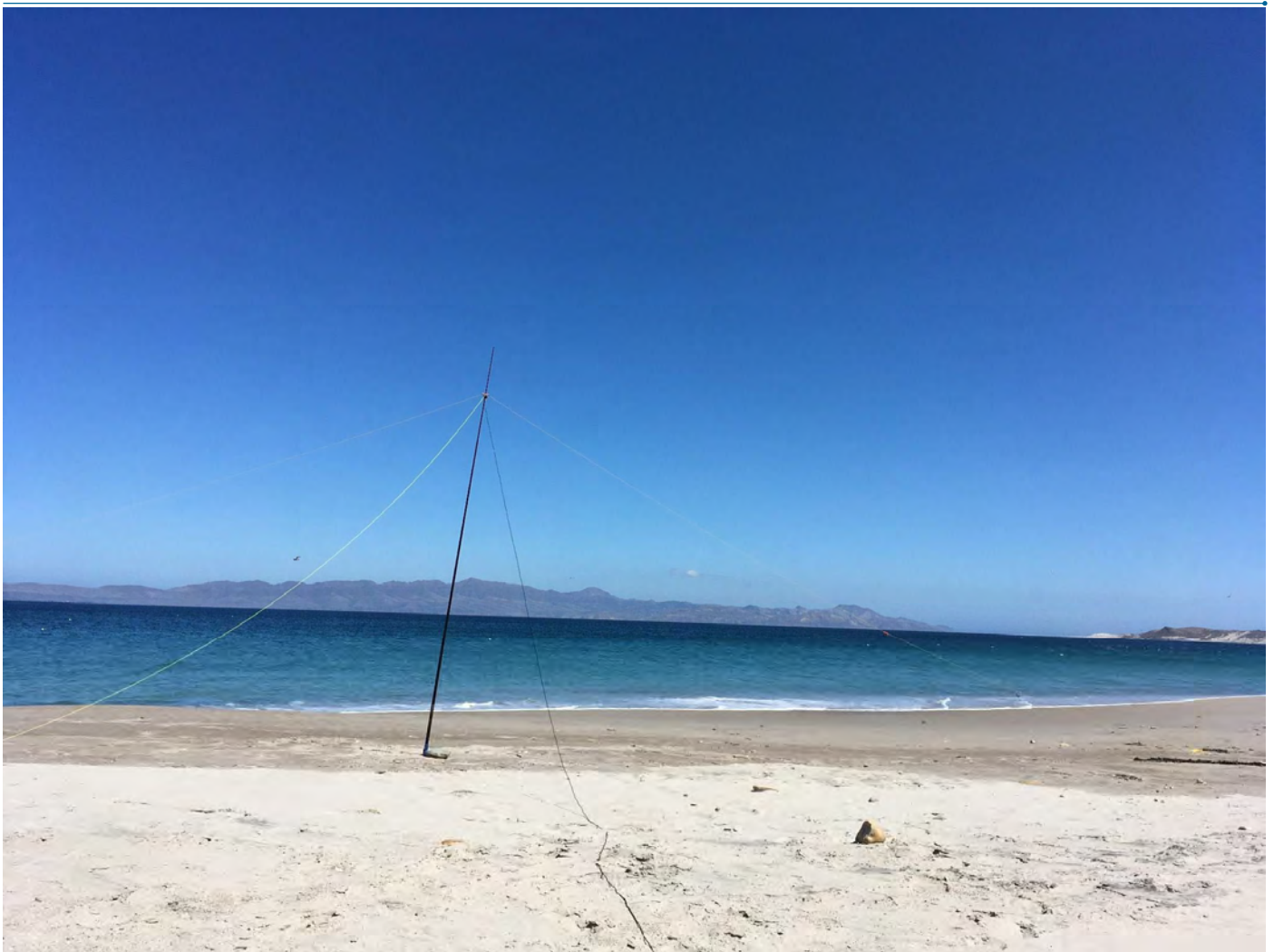
A linked dipole antenna installed on Santa Rosa Island, oriented toward Santa Cruz Island. This antenna supported portable HF operations in a challenging island environment, providing reliable performance while allowing for quick and flexible band changes in the field. Photo by Philomen Leonelli Jr., WM6Y.
