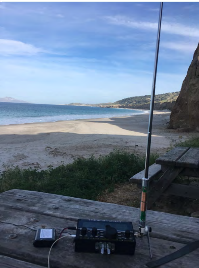
An Elecraft KX2 transceiver deployed on Santa Rosa Island as part of a portable HF operation. The KX2's small size, internal battery options and strong performance made it well suited for island activations and field use. Photo by Philomen Leonelli Jr., WM6Y.
