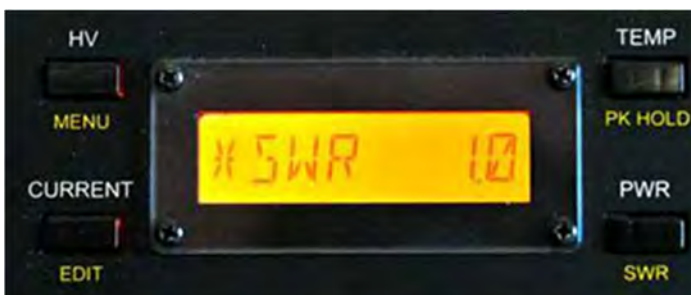
Figure 4. A KPA500 SWR readout of a three-element 6-metre Moxy at 50.313 MHz
