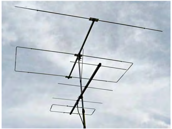
Figure 1. Dave Ahlgren, K1BUK's 6- and 2-metre Moxy antennas on a 4,8 m painter's pole
