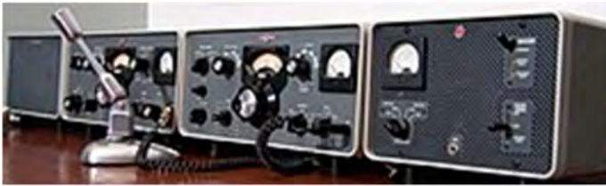
Above. Collins S-Line, featuring separate power supply, receiver, transmitter and speaker console, c. 1960s Right. EF Johnson Viking Ranger transmitter, c. 1958
