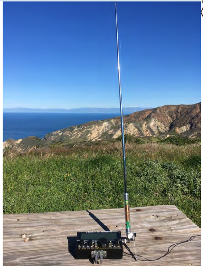
An Elecraft KX2 set up for portable operation on Santa Cruz Island. Photo by Philomen Leonelli Jr., WM6Y.
