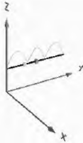
Figure 22: 30 m-band or third harmonic current distribution
