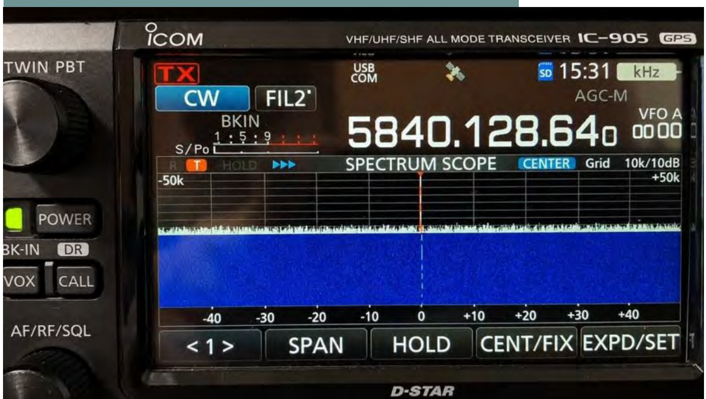
Reception of a 5,84 GHz CW signal from Fuji-OSCAR 126 (FO-126) displayed on an Icom IC-905. [Credit: JA10GZ]
