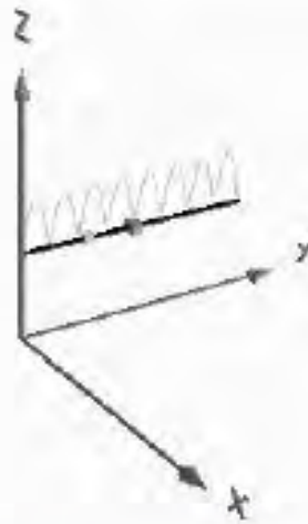
Figure 25: 10 m-band or eighth harmonic current distribution
