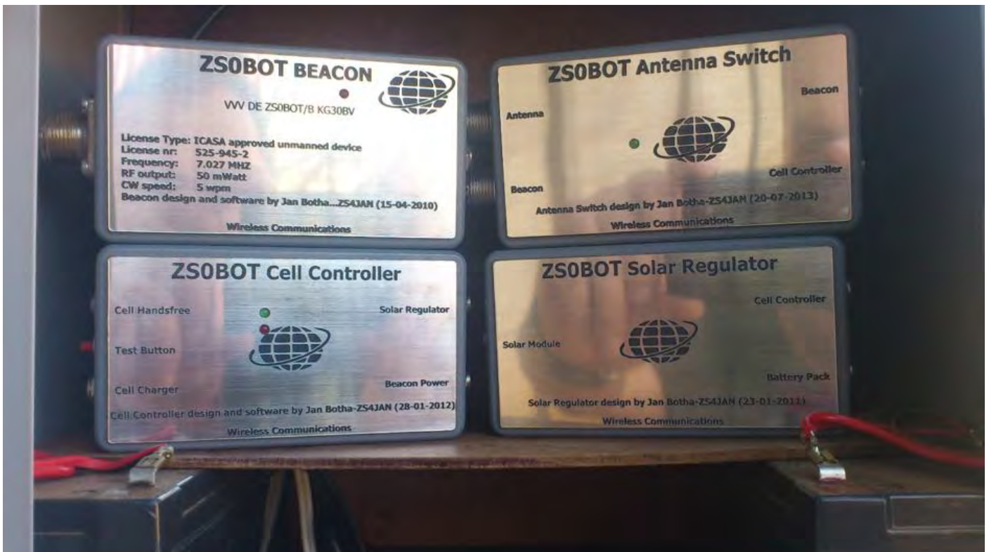
The ZS0BOT/beacon, the Antena Switch, the Cell Controller and the Solar Regulator modules
