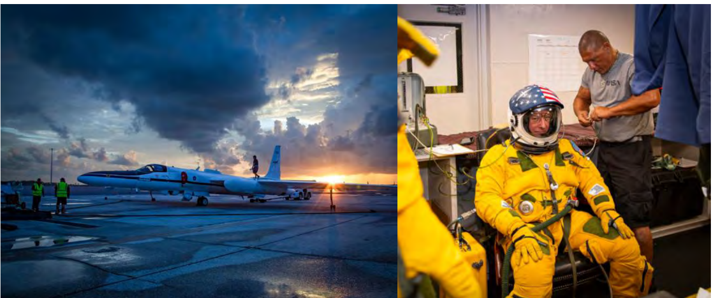
The NASA ALOFT mission used a high-altitude ER-2 aircraft (left) with pilots (right) flying directly over tropical thunderstorms to detect high-energy particles and radiation associated with lightning. NASA/Carla Thomas
