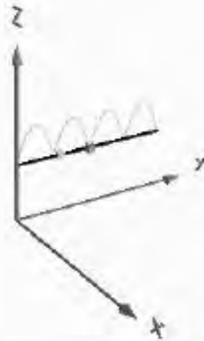
Figure 23: 20 m-band or fourth harmonic current distribution
