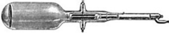
Braun's original cold-cathode CRT, the Braun tube, 1897
