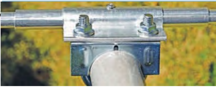
Top. Figure 3. Element-to-boom mounting.
