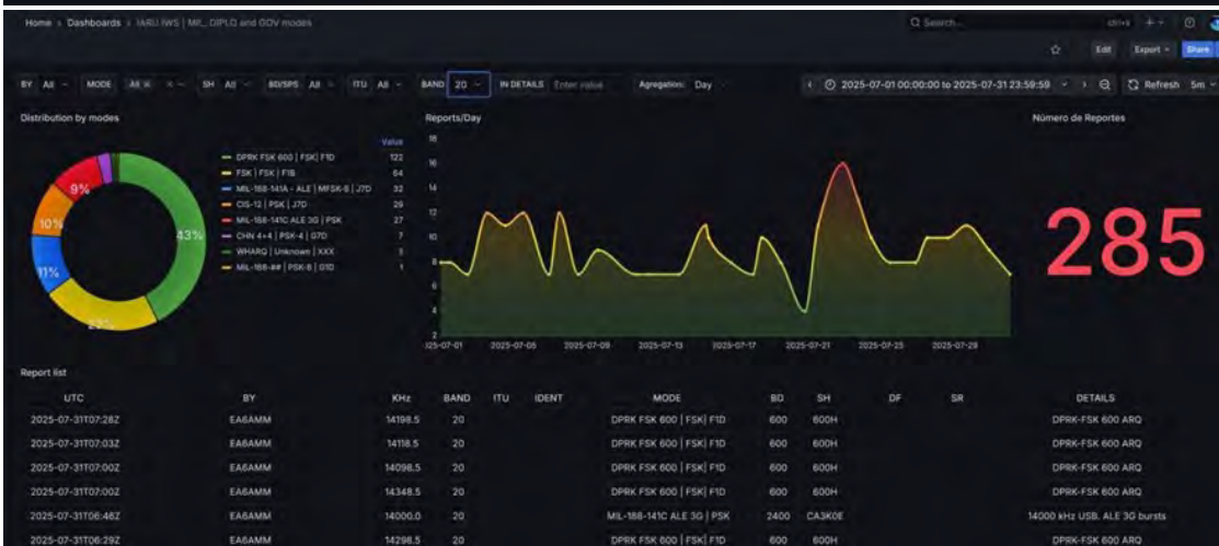
Images 2 and 3: non-amateur transmissions sent in MIL and DIPLO modes on 20 m during July 2025
