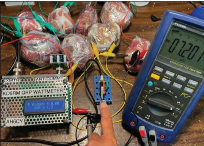
Photo B. This eight-bank tuber array produced 1 mW of power with a current drain of 7,729 mA. (AH6CY photo) Photo C. Shady Brook Farm in Yardley, Pennsylvania, yields from 25 000 to 35 ,000 pounds of potatoes per acre, more than enough for the Lauton Institute’s experiments. 7
