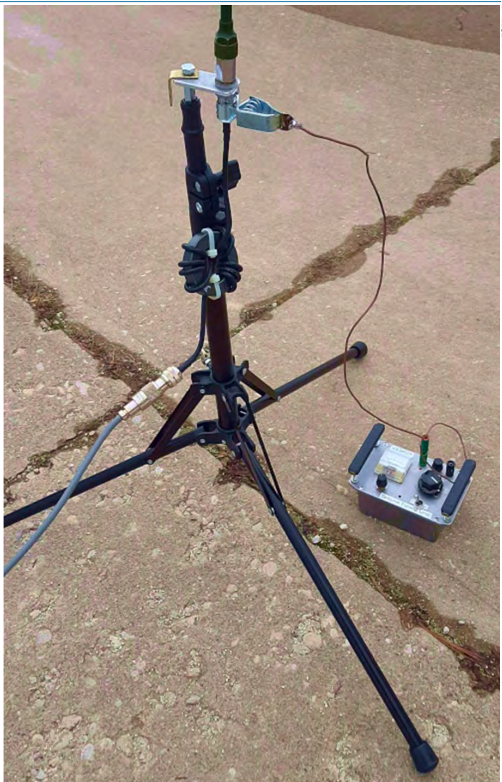
Final setup. This picture was taken before the chicken wire capacitance plate was in place. The antenna was fed by a 10 ft/3 m RG-8 coax through a Common Mode Current choke (on a FT240-31 toroid).
