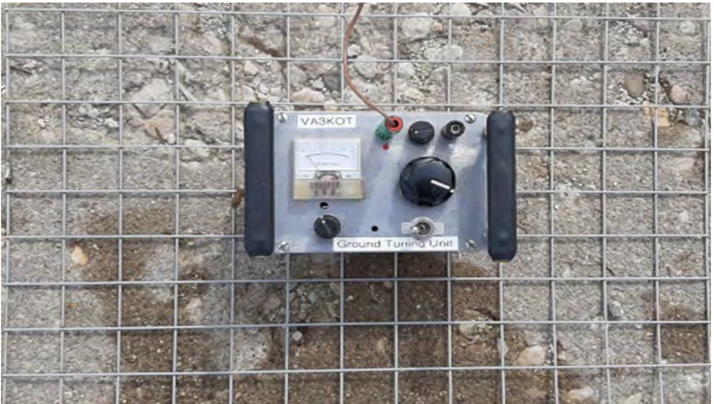
GTU atop its chicken wire capacitance plate. The large toggle switch bottom right is a bypass switch. The knob under the meter selects one of three inductors. The knob at top right adjusts the deflection of the meter needle. The large knob is for the tuning capacitor.
