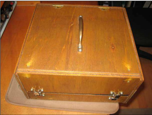
The lid, its hinges and brass handle and view of front two-piece panel with coach clasps.
