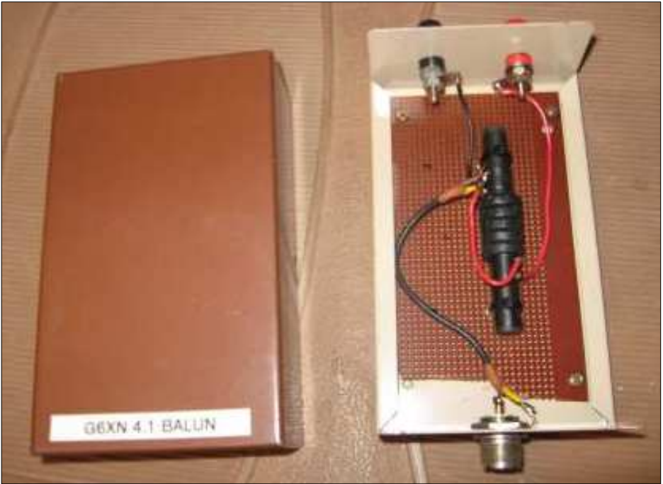
4:1 Balun mounted in a metal enclosure with connectors for coax and 300/450 ohm Window Feed line. Note the use of plain veroboard for mounting. Plain glass fibre pcb board and or thin Perspex can also be used. The veroboard has been mounted on stand-off supports.
