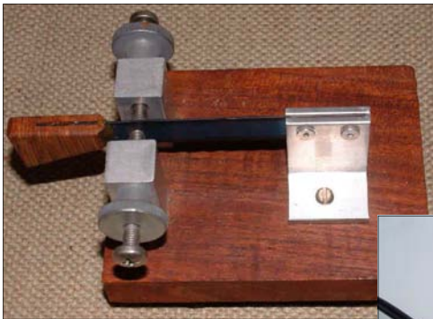
Photo 4. A single lever CW paddle like this popular Begali "Simplex Mono" version can be converted to Sideswiper function by clip lead connecting its left and right contacts together. Alternately, a stereo-to-mono adapter plug installed between paddles' plug and transceivers' socket will change paddle to Sideswiper.
