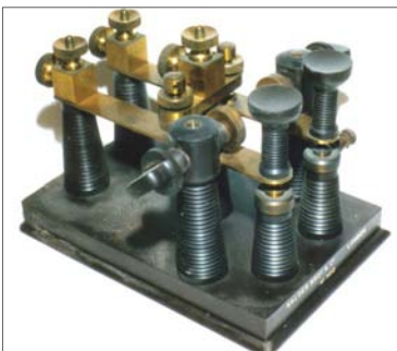
Germany makes this Cricket/iambic "Squeaky" paddle, and its 45-degree-angled arms make sending CW from unusual positions quite enjoyable. Note round finger pieces for vertical, horizontal or angled operation. Details at www.morsekey.com . E-mail insec0.wenk@t-online.de .
